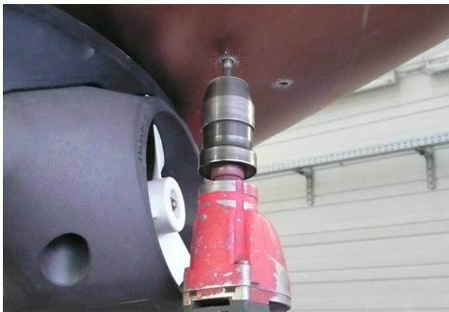
Fig. 19: mounting bolts drilling
