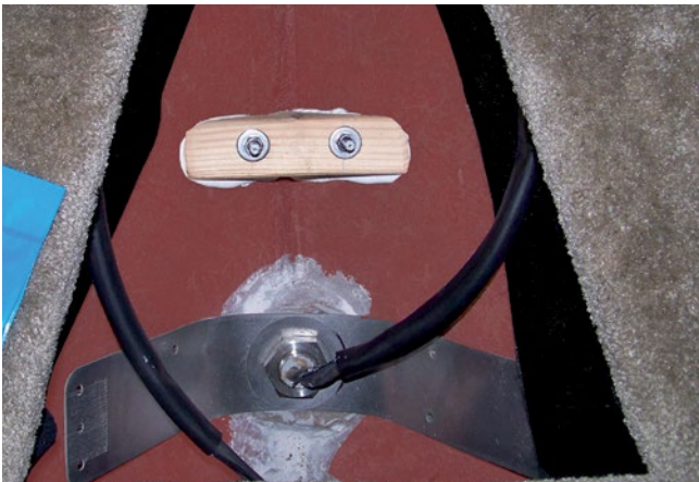
Fig. 25: Screw connection GRP in the boat interior
