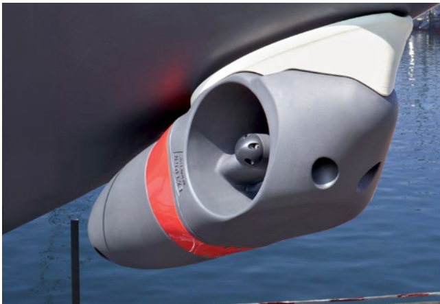
Fig. 22: EX series mounted with mounting kit „Adapter“
