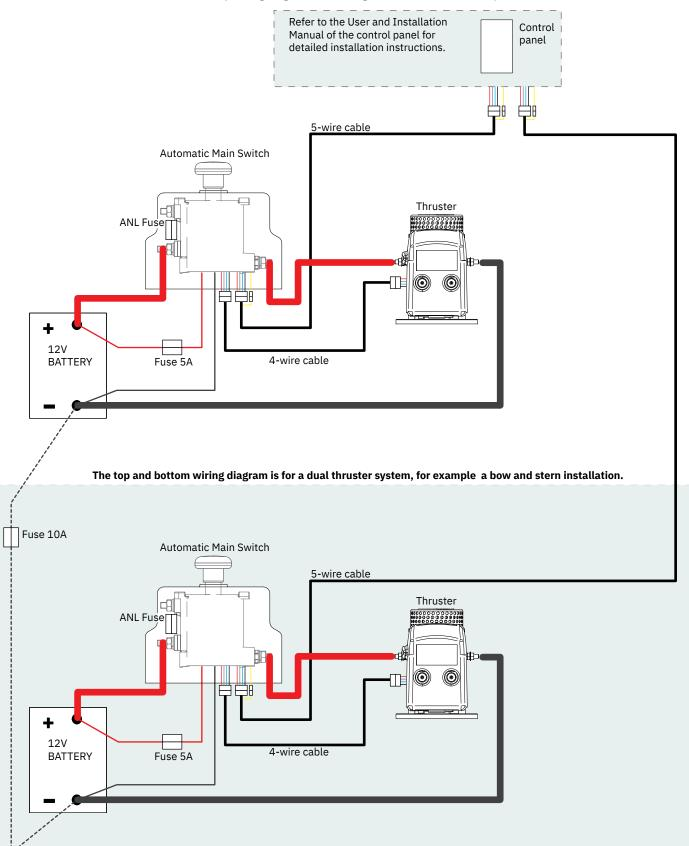
The Top wiring diagram is for a single bow or stern thruster system
