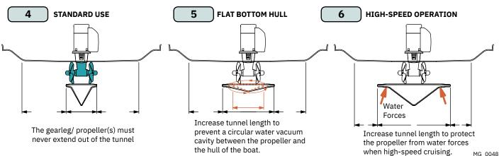
Some sail boats have a flat bottom and shallow draft in the bow section. This can make installing the thruster as far forward from the boats main pivot point difficult.
