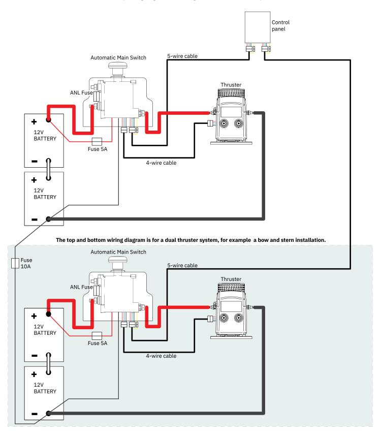
For **Control Panel** installation please refer to the Installation Guide accompanying the control panel to be installed.
