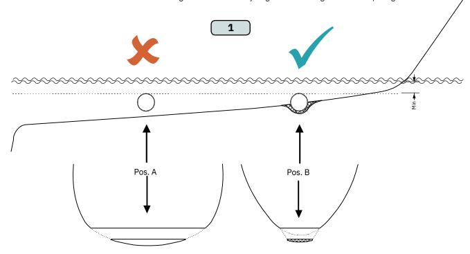
A possible problem in sail boats or fast powerboats is that a non-rounded surface can generate drag from the back face of the tunnel, as it creates
