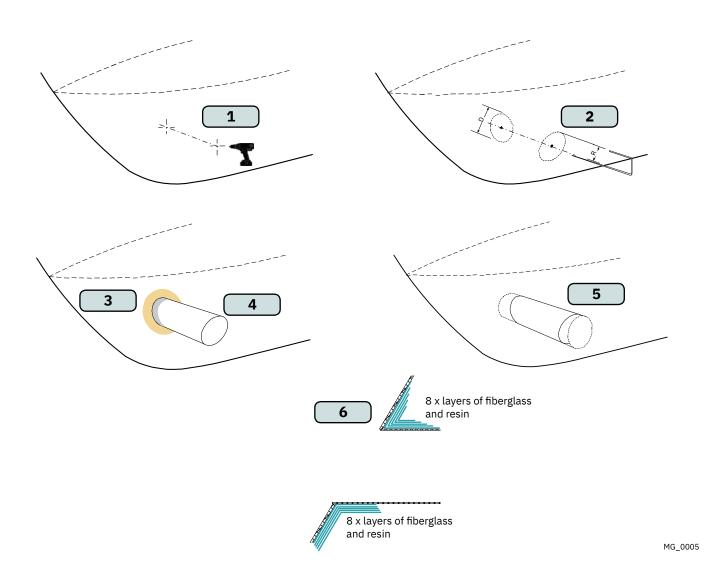
With tunnel installed and cast.
