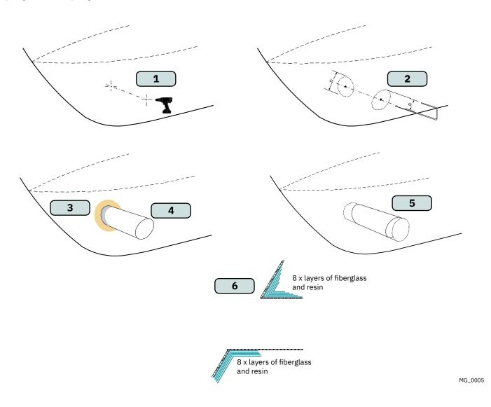
With tunnel installed and cast.
