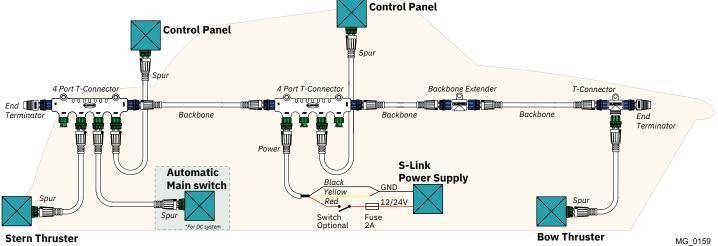
SEP20 & SEP25 & SEP30 & SEP40 5090 - 16 For **Control Panel** installation please refer to the Installation Guide accompanying the control panel to be installed.
