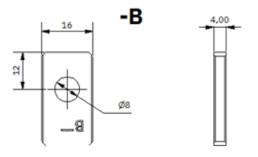
Illustration above shows the dimensions of the two terminals. The only difference is the bolt hole diameter. For the correct installation of the power cables, two different markings/guides have been added.
