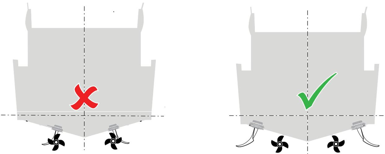
Fins should be placed as far outboard as possible, and NOT in-line with the propellers, to ensure avoiding possible disturbance of the water flow to the props which in the worst case can cause vibrations / cavitation.
