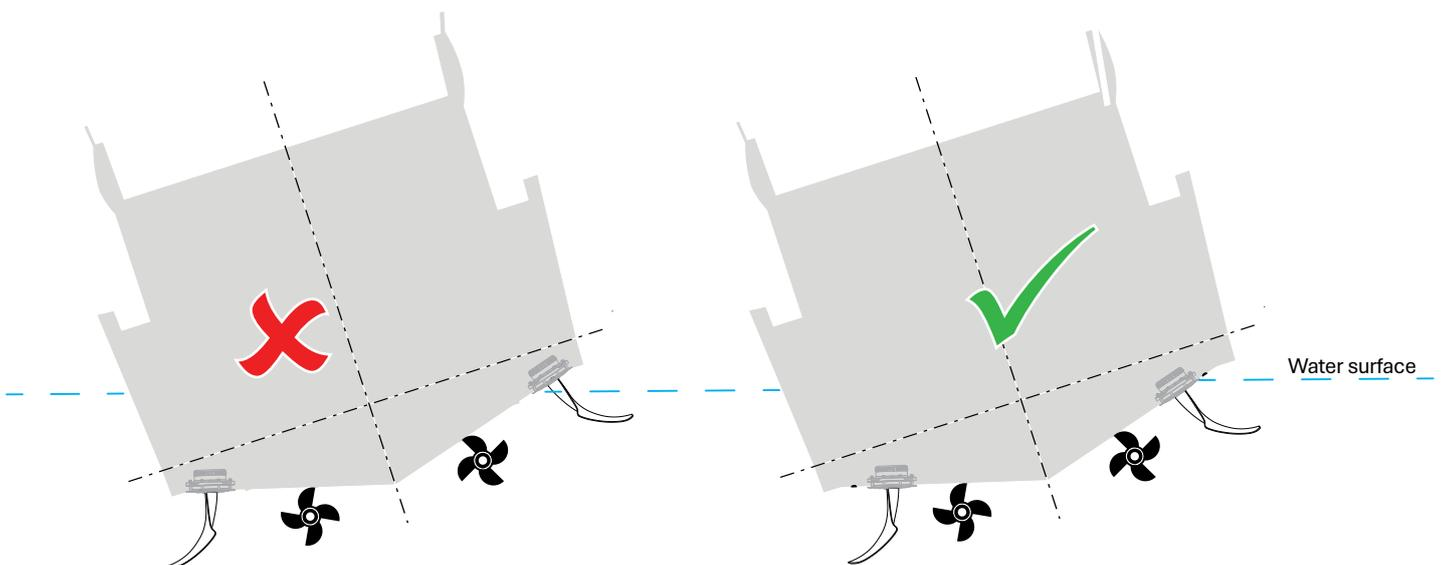
No part of the fin should be above water level during normal roll motion/under normal sea conditions.
