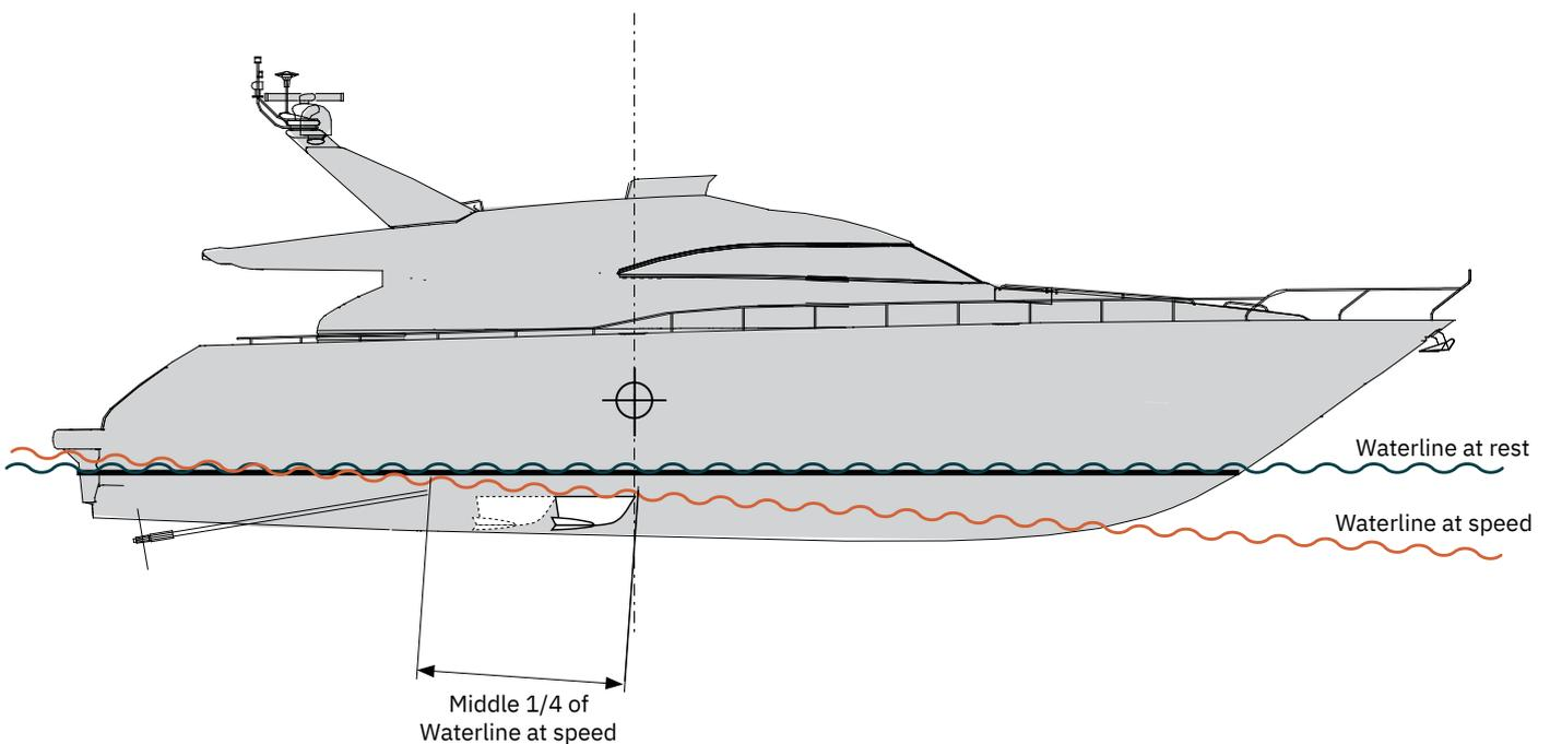
To avoid unwanted influences on the steering characteristics, the fins should be placed close to the vessel longitudinal centre of gravity (LCG)
