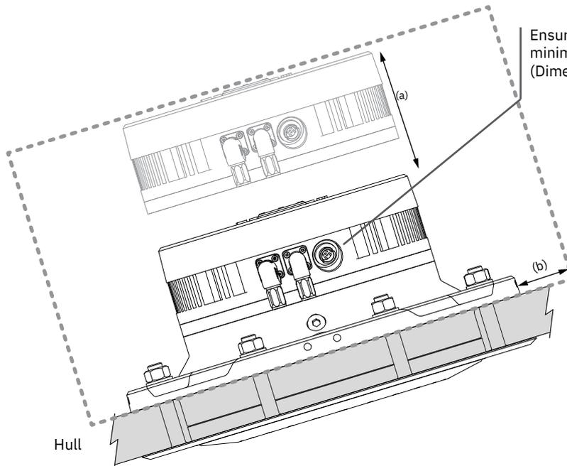
Ensure enough space around the actuator to obtain the specified minimum bending radius of 151713-xxx (SCU) cable. (Dimension code (c)).
