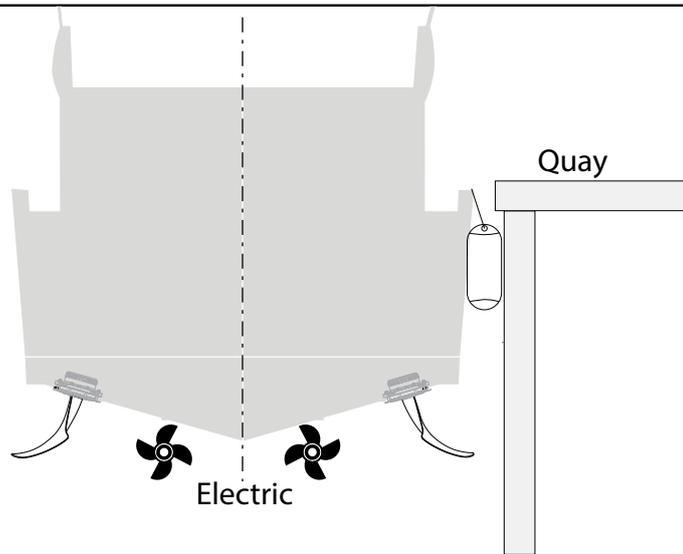
Fins should not extend outside the beam including the fenders, or below the keel/propeller when in neutral position.
