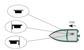
The control unit should be mounted in an upright position. The label on the front side is marked with an UP arrow that should point upwards and a FWD arrow that should point in the forward direction. Exact mounting is not critical, however, as the desired running attitude is set after installation.
