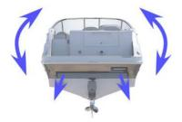
ACS A automatically adjusts the boat to the optimum attitude in the pitch axis, improving visibility and also enabling speeds in the "semi-planing" range. It also improves the "hole shot".
