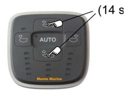
The AUTO indicator blinks to indicate that calibration is needed. Press the uppermost and lowermost buttons simultaneously for 5 s to start the calibration. Keep the buttons depressed for another 9 s, while the ACS is calibrating.
