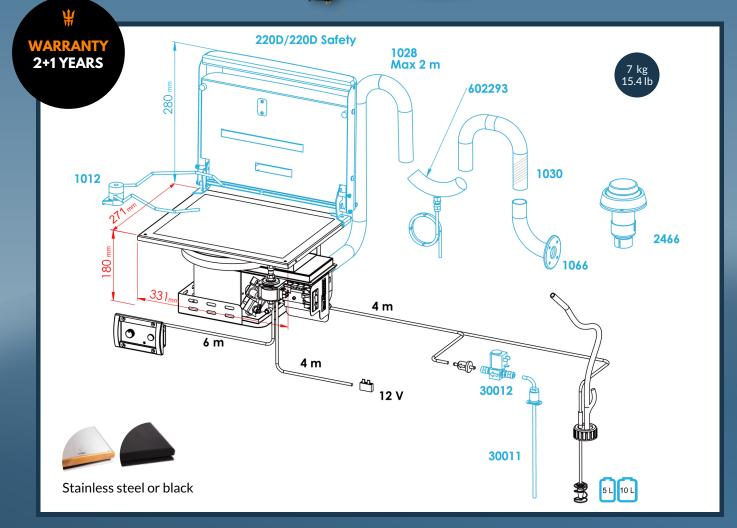
Accessories in black come with the standard package. Accessories in blue are additional/optional. The calculated values are measured in a reference measurement wall, which is constructed to represent a typical boat installation. The figures allow for 10 % reserve - yours may vary.
