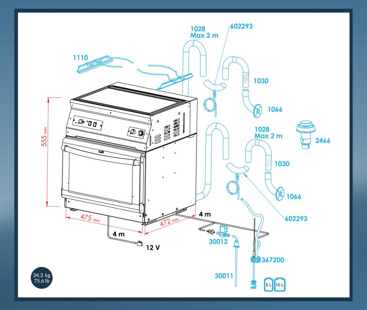
Accessories in black come with the standard package. Accessories in blue are additional/optional. The calculated values are measured in a reference measurement wall, which is constructed to represent a typical boat installation. The figures allow for 10 % reserve - yours may vary.
